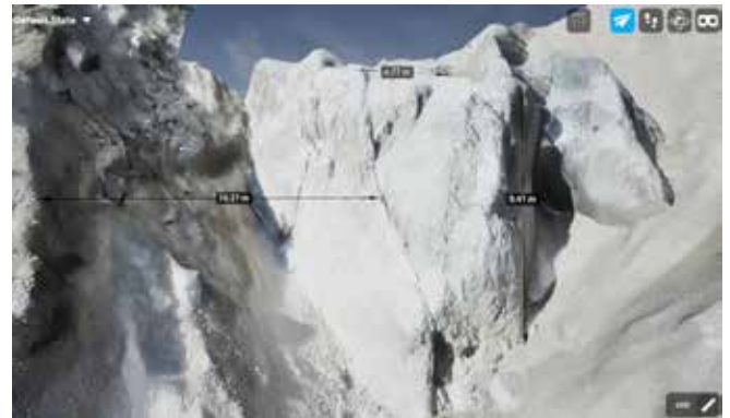
Fig.5. Example of the measurement functionality applied to the monolithic boulder in the Cancia channel.
