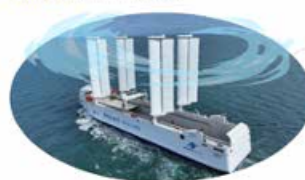
Fig. 1. The challenge of optimizing wind propulsion at sea. This real photograph shows a vessel equipped with four Oceanwings, surrounded by different wind directions. It highlights the combinatorial complexity of optimizing performance at sea.
